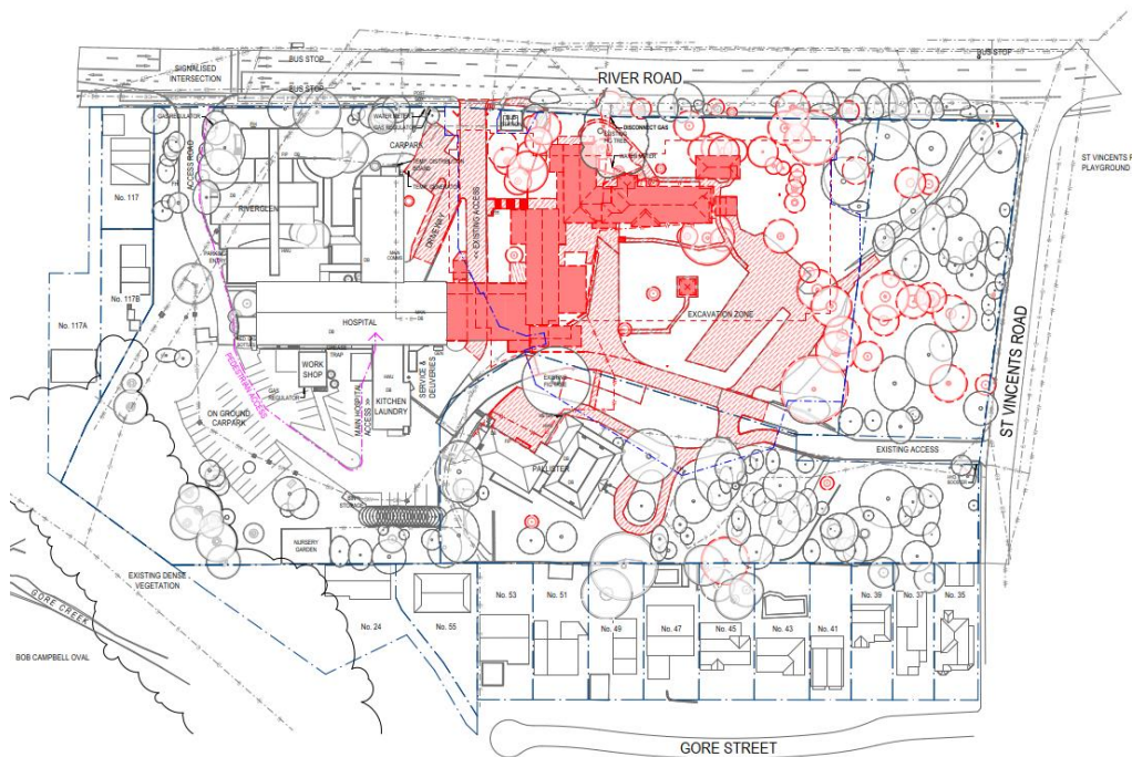
Figure 2 - Demolition for Stage 2
